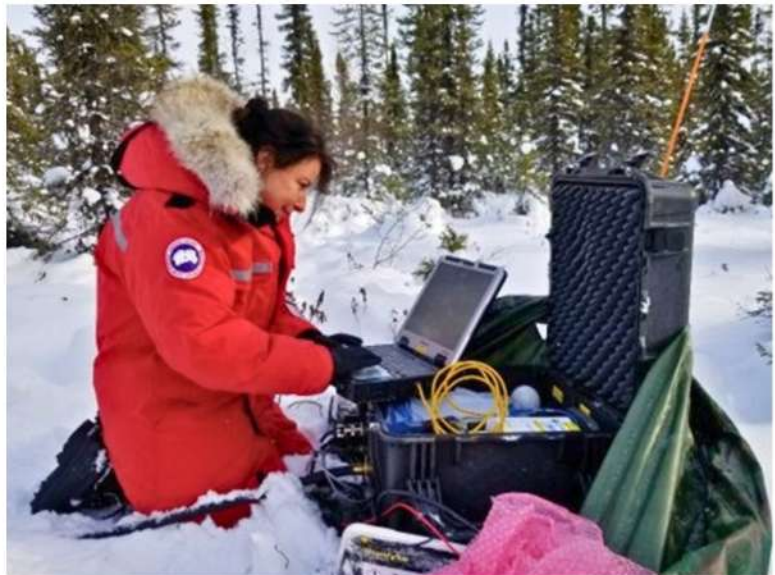
NRCan Research Scientist Dr. Claire Perry installs a temporary seismic station for a noise study in Labrador
